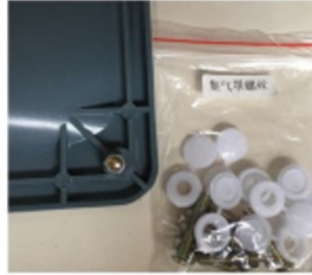
2. Gas collecting hood and related screw fittings
