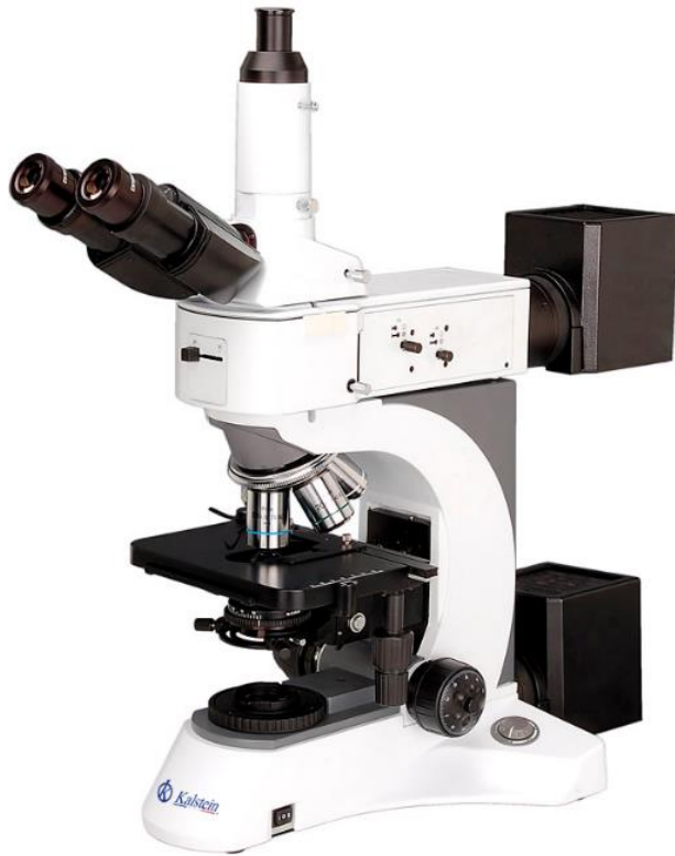
Seidentopf Trinocular Head, 30° Inclined, Interpupillary 48~75mm Extra Wide Field Eyepiece EW10x/22mm, Eyepiece Tube Dia.30mm
